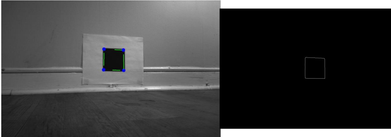
Figure 1: The original image with the lines output from the RANSAC like algorithm shown in green and the points designating the corners shown in blue, along with the edges output from the Canny edge detector.
