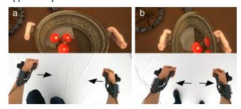
Figure 7. Wearing PIVOT on both arms enables haptic feedback for bimanual interactions. Here, the user is stretching and compressing a basket, which is rendered as synchronized push-pull forces on both hands.
