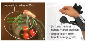
Figure 14. When reaching out to pick up an object, PIVOT checks the distances to the surrounding objects. If an object is in the 30cm radius, the handle moves to the preparation position with moderate speed. When the target distance becomes closer than 10cm, the handle starts to move continuously closer to the hand with the decreasing distance.
