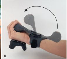
Figure 1. PIVOT is a wrist-worn haptic device with a pivoting handle that appears in the user's hand on demand, rendering grasping, catching, and throwing hand held objects in virtual reality.
