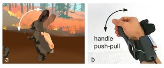
Figure 6. The user feels the inertia of the wiggling bunny through PIVOT's handle being actuated back and forth.
