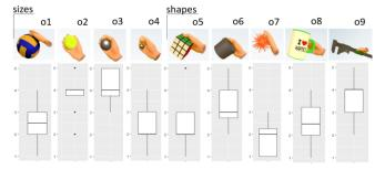
Figure 15. Task 1: Grasping objects of different shapes and sizes. We presented participants with: (o1) a big ball larger than PIVOT's grip (12cm), a (o2) tennis ball (7 cm), (o3) a ball about the size of PIVOT's grip (5cm), and (o4) a small ball (1.5cm). Additionally, participants interacted with: (o5) a Rubik's cube (7cm), (o6) a cylinder (7cm), (o7) a spiky sphere (7cm), (o8) a mug (2cm handle), and (o9) a wrench (4cm handle).
