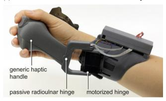
Figure 2. PIVOT's key design element is the actuated pivoting handle that is grounded to the user's forearm.
