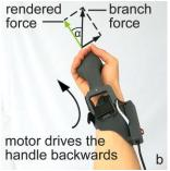
Figure 5. PIVOT renders the normal component of the springy force of the branch by actively driving it's handle while being grasped.
