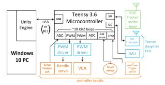
Figure 10. PIVOT's system diagram
