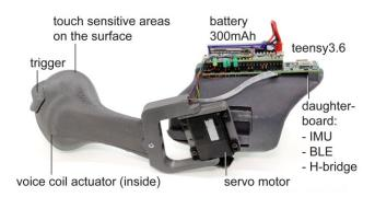
Figure 9. PIVOT's functional elements: touch sensors, voice coil actuator (VCA), Teensy microcontroller with H-bridge daughterboard, and a retrofitted RC servo motor.
