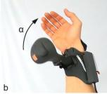
Figure 3. (a) When reaching out for a virtual object, (b) PIVOT rotates its handle towards the user's hand inverse-proportionally with the distance to the virtual object.
