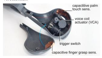
Figure 13. The inside of the handle contains: a trigger switch, capacitive touch sensing copper tapes, and a VCA.
