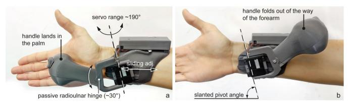
Figure 11. PIVOT's mechanical design: the servo actively pivots the handle around the slanted vertical axis, while the handle affords passive radioulnar motion to accommodate natural hand tilting. A sliding rail mount on the hand-cuff enables adjustment to individual hand sizes.
