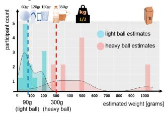
Figure 19. Results of task 3: Participants subjective weight estimation for the lightest and the heaviest ball (dotted lines shows the weight PIVOT rendered)
