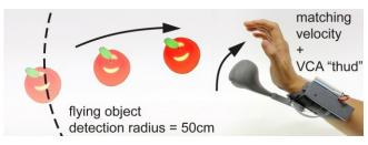
Figure 4. When an object is detected approaching the user's hand with a higher velocity than 0.5m/s, PIVOT predicts the moment of contact and starts moving its handle early on to produce a haptic collision sensation at the right moment.
